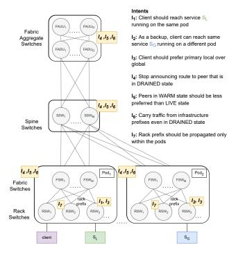
Figure 1: Data center topology with sample intents.
