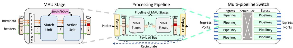
**Figure 1: PISA-based switch, adapted from RMT architecture [7]. We show the switch in different levels of detail: Match-Action Unit (MAU) stage within a single switch pipeline (left), switch pipeline of MAU stages (middle), and a switch with multiple pipelines (right).**
