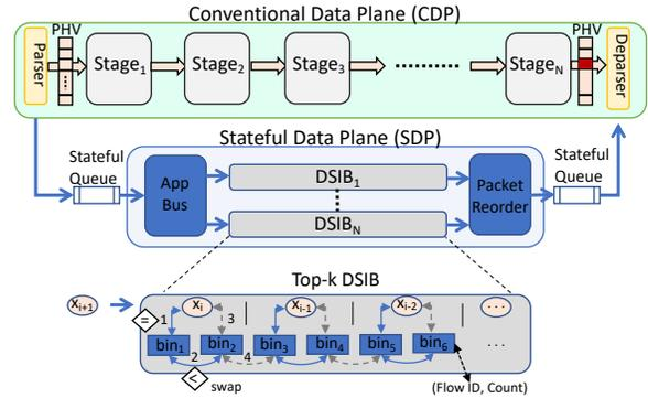
**Figure 2: Our vision for the next generation of programmable switches is a Stateful Data Plane (SDP) that computes the state while packets traverse the Conventional Data Plane (CDP). Individual stateful computations can be implemented through specialized blocks (DSIB). We show in the detail how a DSIB calculates the top- $k$  flows using a pipelined hardware algorithm [45].**
